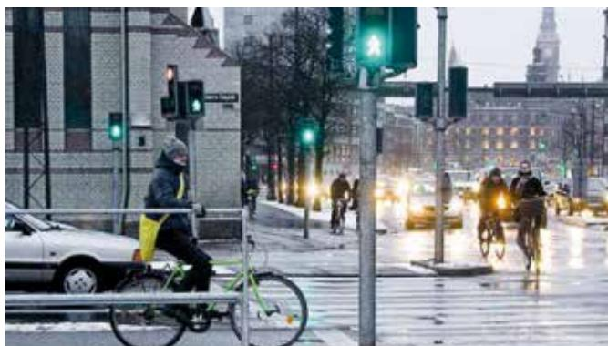
**Figure 29. Junctions – resting rails provide support and convenience at junctions and have been implemented in Copenhagen, DK and are starting to appear in other cities such as Chicago, USA (Photo: Copenhagenize.com)**
