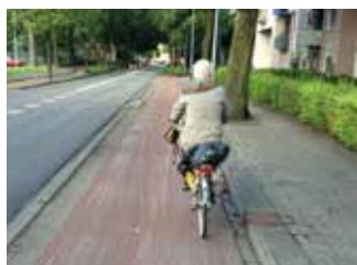
**Figure 30. Separated Cycle Paths – the Netherlands uses red colour and texture on its cycle paths throughout the country so inhabitants are clear on the distinction between cycle paths and pedestrian paths. (Photo: Tim Jones)**
